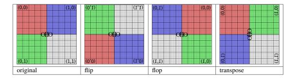
ImageBuf 0IIO::ImageBufAlgo::reorient(const ImageBuf &src, int nthreads = 0)
